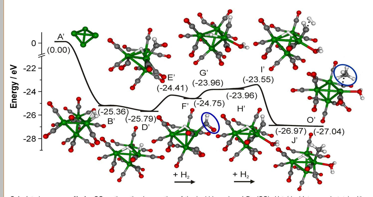
Calculated energy profile for CO methanation by reaction of the hydrido carbonyl Ru<sub>4</sub>(CO)<sub>13</sub>H<sub>2</sub>+ (doublet ground state) with two sequentially adsorbed H<sub>2</sub> molecules together with the corresponding structures. The numbers indicate the relative energies in eV. The blue circles highlight the formyl-type intermediate in structure F' and the final methane product in structure O' [4].
