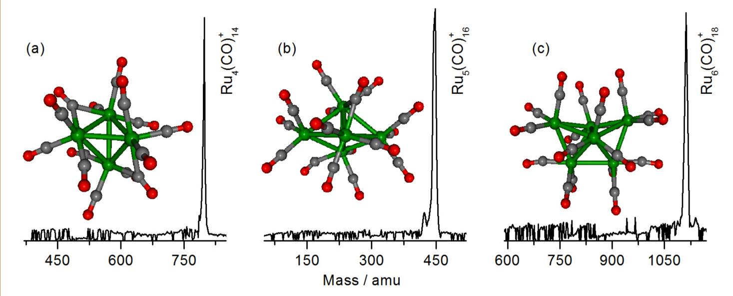
Product mass spectra obtained after reaction of (a) Ru<sub>4</sub>+ (b) Ru<sub>5</sub>+ and (c) Ru<sub>6</sub>+ with CO for a reaction time of 0.1 s. Also displayed are the corresponding DFT structures of the most abundant products. Ru, C, O and H are indicated by green, gray, red, and white spheres, respectively [3, 4].
