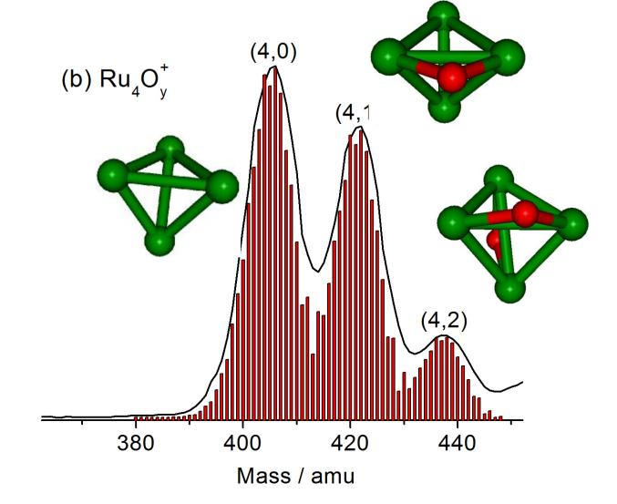
(b) Enlarged view of the cluster signal in the mass range between 380 and 450 amu. The bars represent the calculated mass distribution of  $Ru_4O_v^+$  (y = 0 - 2) derived from the natural abundance of the ruthenium isotopes.
