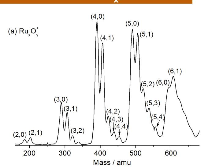
Ruthenium and ruthenium-oxide distribution generated by the CORDIS sputter source. The mass peaks are denoted with (x,y) corresponding to complexes of the stoichiometry Ru<sub>x</sub>O<sub>v</sub><sup>+</sup>.
