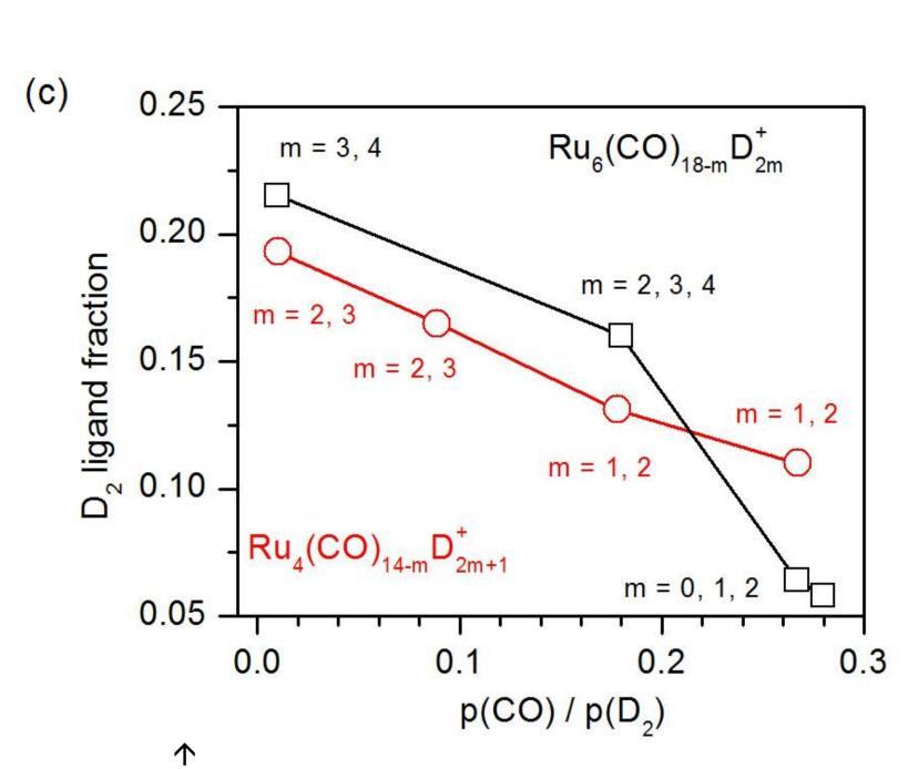
(c) D<sub>2</sub> ligand fraction (average number of D<sub>2</sub> molecules normalized to the total number of ligands in all observed complexes  $Ru_4(CO)_{14-m}D_{2m+1}^+$  and  $Ru_6(CO)_{18-m}D_{2m}^+$ , respectively) as a function of the CO/D<sub>2</sub> partial pressure ratio. Next to each data point the numbers m of the observed coadsorption products are given. The solid lines are drawn to guide the eye [4].
