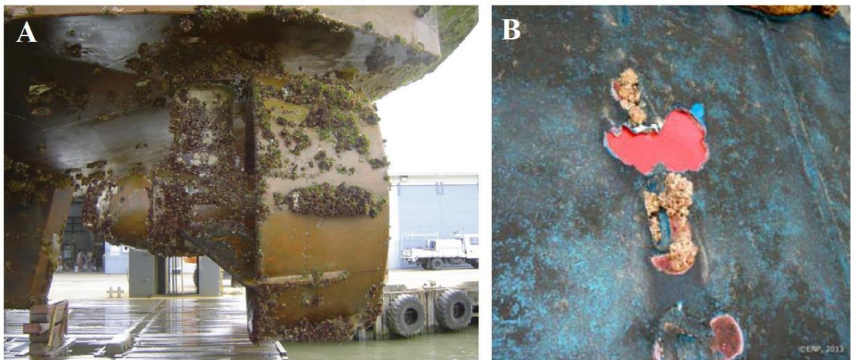
**Figure 2.** A) Vessel hull fouling [14] B) Biocorrosion [15].
