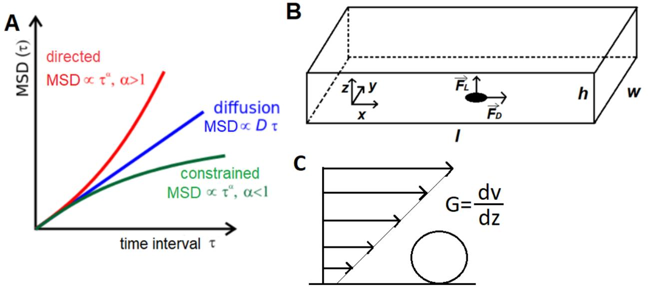
**Figure 6.** A) MSD dependence of time interval  $\tau$  for diffusion (proportional to  $\tau$ ) and directed or constrained motion. B) Rectangular microfluidic channel defined by the width  $w$ , height  $h$ , and length  $l$ , with specified axes. A bacterium adhered at the surface is shown with drag and lift forces that act upon it. C) A schematic representation of the shear rate of ambient flow  $G$ .
