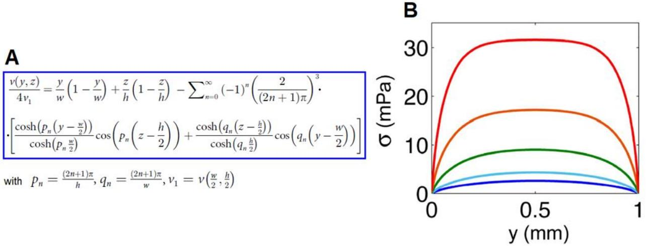
**Figure 7. A)** Velocity field calculation for a steady viscous flow of an incompressible fluid in a rectangular channel [52]. **B)** Bottom shear stress variation across the channel width as a result of velocity field  $v(y, z)$ , given for 5 rectangular 1mm-wide channels, ranging in height from 250  $\mu\text{m}$  (red) to 1000  $\mu\text{m}$  (dark blue), under a flow rate of 1 ml/h [52].
