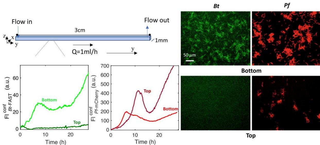
**Figure 5.** A schematic view of millifluidic channel together with surface-dwelling characteristics of two different species, both at the bottom and the top, measured as confocal fluorescence intensities [55].
