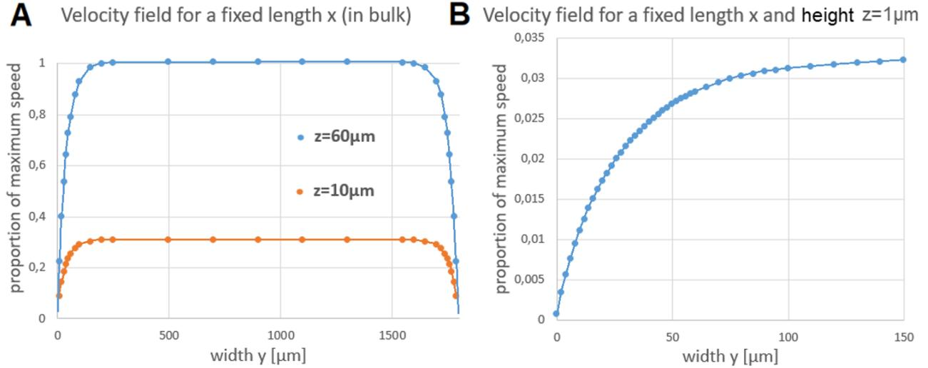
**Figure 8.** **A)** Velocity field at a fixed  $x$  position and at the heights of  $z = 60\mu\text{m}$  and  $z = 10\mu\text{m}$ , in a  $1.8\text{ mm}$ -wide and  $120\mu\text{m}$ -high channel. **B)** Velocity field at the height of  $z = 1\mu\text{m}$ , at which the bacteria is situated while adhered at the surface.
