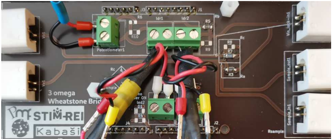
Figure 3.4: Fabricated bridge PCB front view used in the measurements. The balancing branch includes the two series photoresistors marked Ldr1 and Ldr2 and the connection for the external precision potentiometer.
